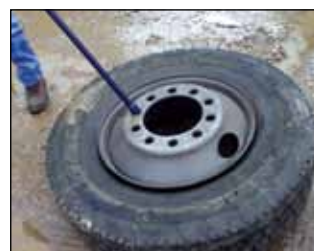
With hub side up insert the knob end
