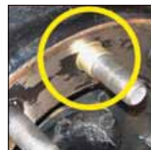
Corrected with centering sleeve
