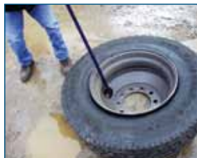
With hub side down use the curved end
