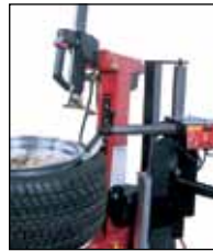
Bead depressing tool aids in demounting
